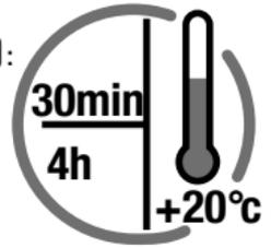
Drying time depends on film thickness and we recommend drying overnight. Drying times in cold temperatures can be longer and applying in cold temperatures might affect the film quality. Thick film can demand a longer time to cure. Final hardness of the coating will be achieved after approximately 2 days.
